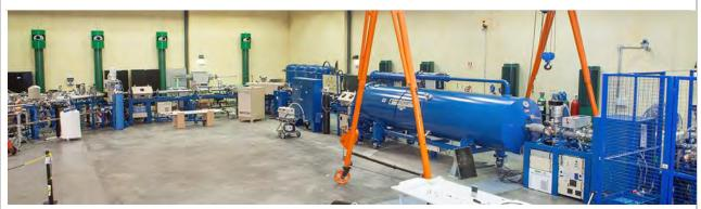
When a sample is exposed to an ion beam, different atomic and nuclear processes are induced. As a result of these processes, several products are generated, and each product provides information on the properties of the material (composition, structure, etc.)
